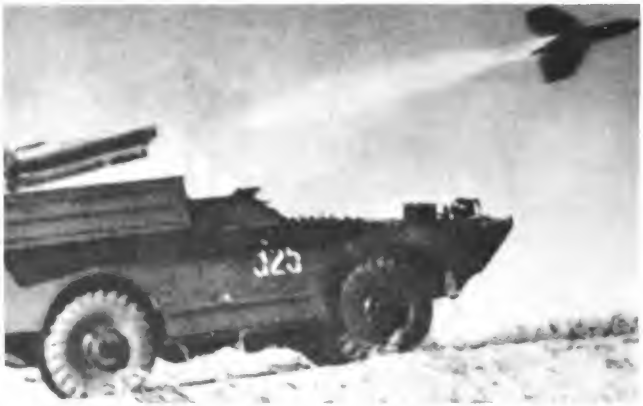
Figure 6-38. AT-3 SAGGER. The newest anti-tank guided missile is the SAGGER, which appears in a six-missile mount on modified BRDM vehicles (above), in a single launcher on many BMP APCs, and in a man-pack ground-fired version (below).
